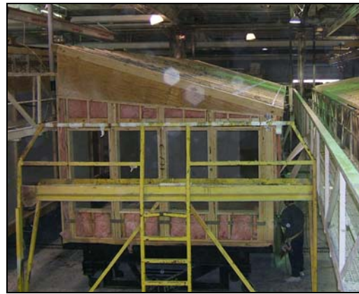
Figure 35 Palm Harbor HUD Code Manufactured Housing factory – production line.
