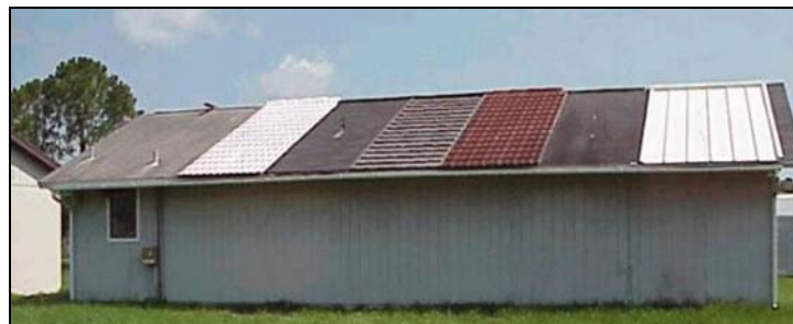
Figure 92 2001 Experimental roof cell. Cells are numbered from left to right starting with the cell second in from the left.
