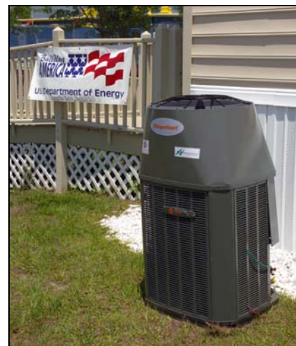
Figure 84 Final test prototype with diffuser and fan.
