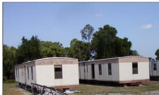
Figure 68 The test units in place. Note white ground cover under unit on left, exposed dirt under unit on right.
