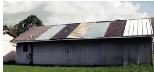
Figure 90 Flexible Roof Facility in summer 2002 configuration. Cells are numbered from left to right starting with the second cell in from the left.
