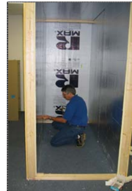
Figure 95 Return Air Flow Test Chamber
